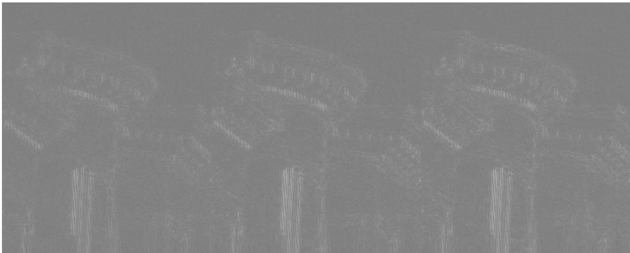
(k) Difference image between the captured DVCPRO HD image (e) and the original source image (a) for the windowed region.
